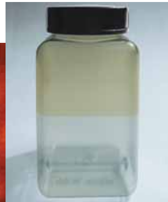
Yellowing: ordinary plastic bottle, upper half exposed to "sun test" for 250 hours
