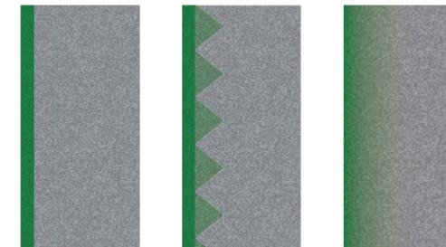
Silicification principle: KEIM Veramin® forms an insoluble bond with the substrate.
