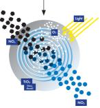
The catalyst titanium dioxide is not consumed. As long as the crystals are supplied with energy by electromagnetic waves (light), the process remains active.
