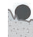
Large areas of the reinforcement are close or right at the concrete surface
